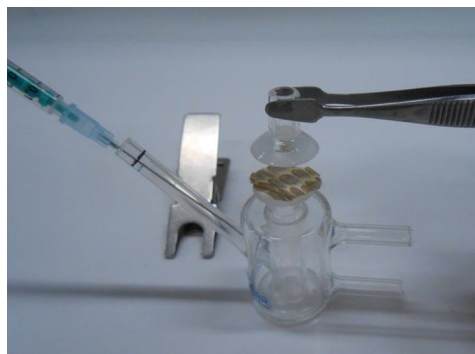
Fig. 1 Photograph of Franz Diffusion cell with a shed snake skin between the donor and receptor parts
