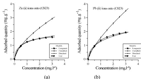
Fig. 2 Langmuir adsorption isotherm at 22°C onto (10 g.l<sup>-1</sup> CKD) (a) Zn (ii) ions (b) Pb (ii) ions
