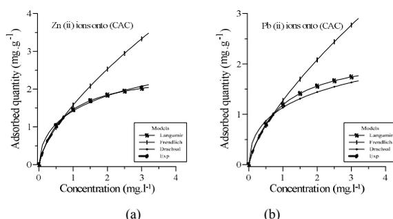
Fig. 3 Langmuir adsorption isotherm at 22°C onto (10 g.l<sup>-1</sup> CAC) (a) Zn(ii) ions (b) Pb (ii) ions
