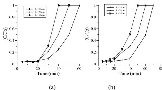
Fig. 1 Breakthrough curves for the removal of Fe (iii) on CKD for different bed heights (a) Fe (iii) on for different bed height  $Q_v=10$  ml/min.,  $C_o=86.6$  mg/l, (b) Fe (iii) on CKD for different bed height  $Q_v=5$  ml/min.,  $C_o=86.6$  mg/l
