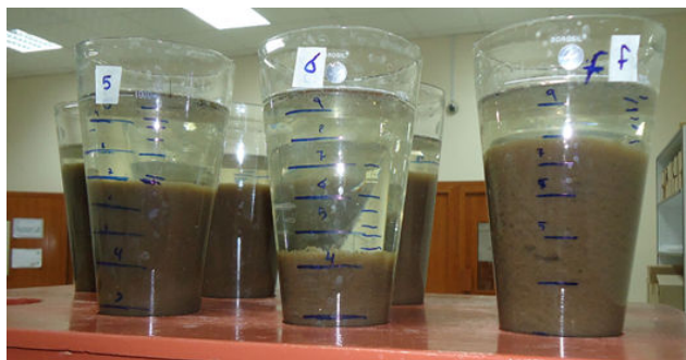
Fig. 1 Effect of Polyelectrolyte concentration on turbidity after 2 hours of settling using same pH value
