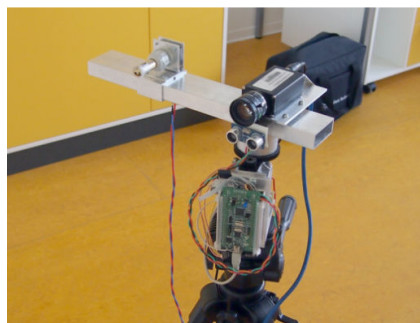
Fig. 1 The laser optical rangefinder
