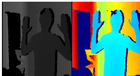
Fig. 6 Plain Depth Data (Left) and Processed Depth Data with RGB Values (Right)
