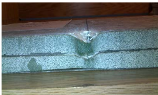
Fig. 5 Cross- section of multi layer sandwich specimen (Sv4) after quasi- static perforation
