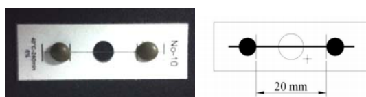
(a) Kenaf bast fiber test frame (b) Specimen dimension schematic diagram
