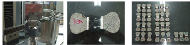
Fig. 8 JCI SF-8 dog-bone test of specimens
