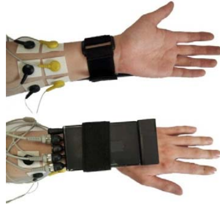
Fig. 4 Sensor modules and the EMG sensor attachment
