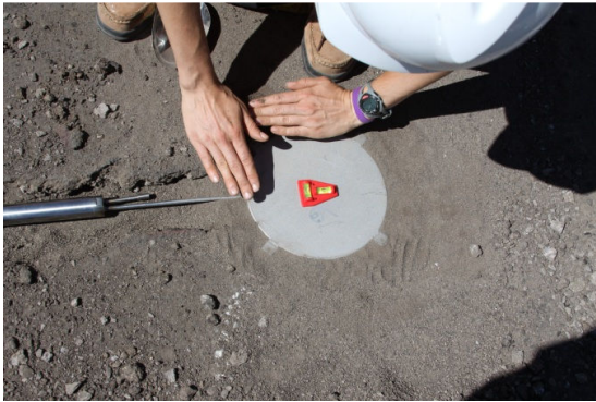
Fig. 4 Installation of earth pressure cell
