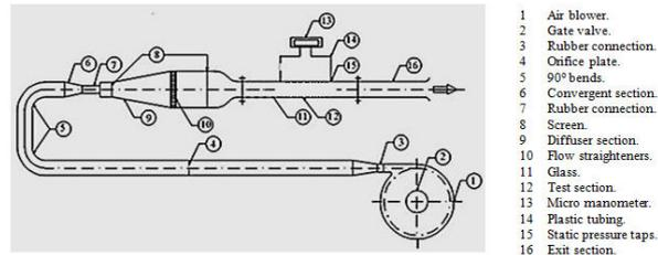
Fig. 1 Schematic diagram of test rig and instrumentation
