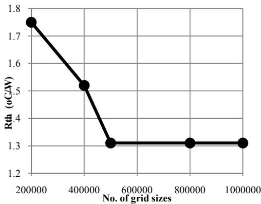
Fig. 3 Thermal resistance at different grid sizes
