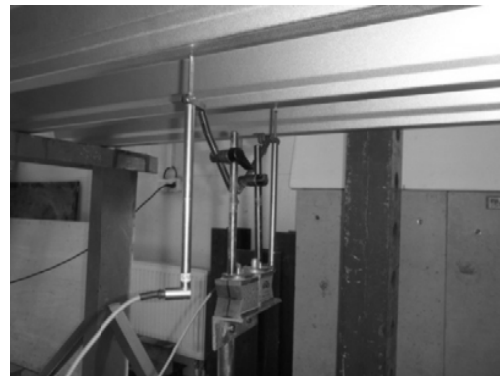
Fig. 9 Measuring instrument on the bottom of the wave sheet
