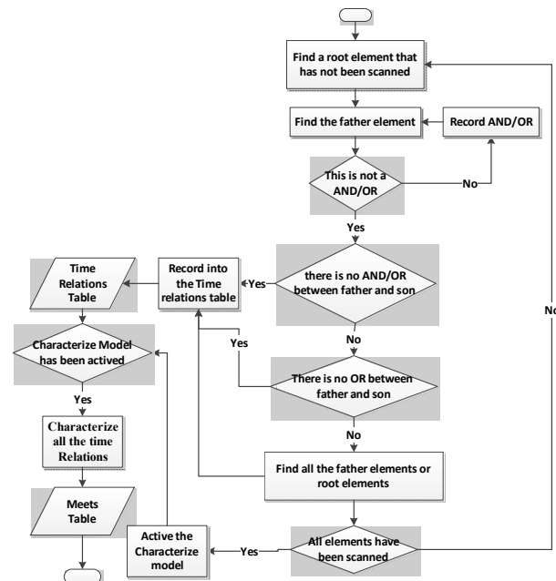
Fig. 8 Flow Chart of TRD Processing
