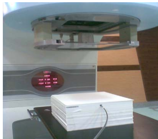
Fig. 2 placement of Tissue equivalent phantom on a flat linear accelerator
