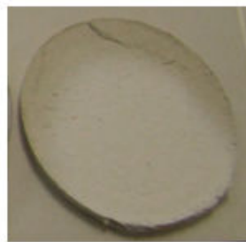
Fig. 5 Underside of the delaminated coating from sample TC1600
