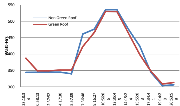
Fig. 8 Air conditioning energy consumption profile for 4th March 2013
