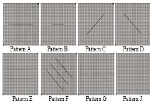
Fig. 2 Glass micromodels used as porous media
