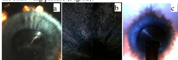
Fig. 12 Several patterns of liquid explosive dispersing flow. a: Inertial dispersion; b: Turbulent dispersion; c: Mixture of inertial and turbulent dispersion
