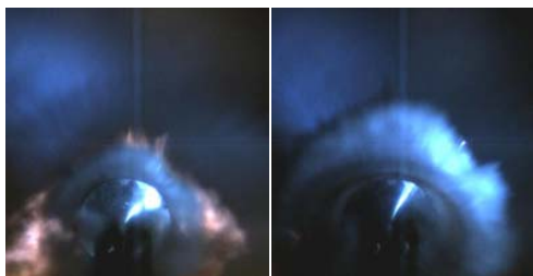
Fig. 10 The shape of water dispersion flow, the explosive charge is 29.3g, the diameter of cylindrical film is 145mm
