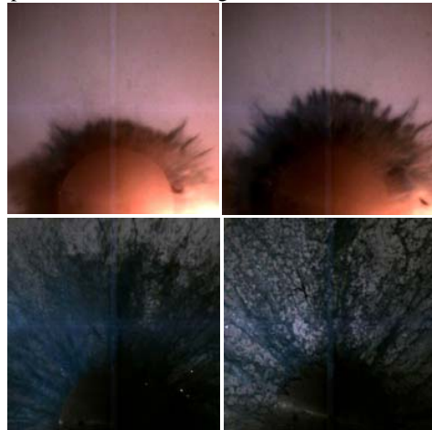
Fig. 5 The shape of water dispersion flow, detonation cord is 3\text{g} \cdot \text{m}^{-1} , the diameter of cylindrical film is 150mm
