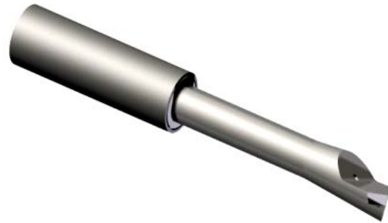
Fig. 5 CAD model of the boring bar
