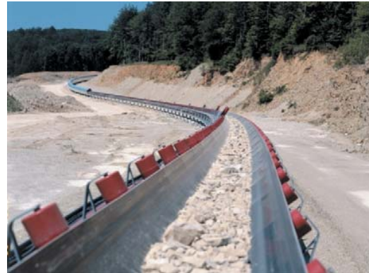
Fig. 1 Conveying limestone material on curved belt conveyors [12]
