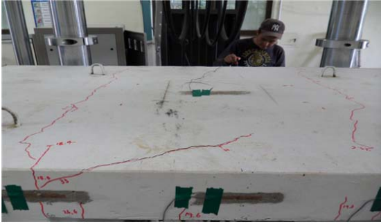
Fig. 11 Crack in ST Type
