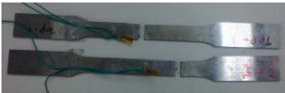
Fig. 10 Broken rail test coupons after tensile test
