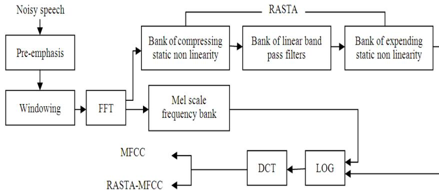
Fig. 1 Block diagram for extracting MFCC and RASTA-MFCC
