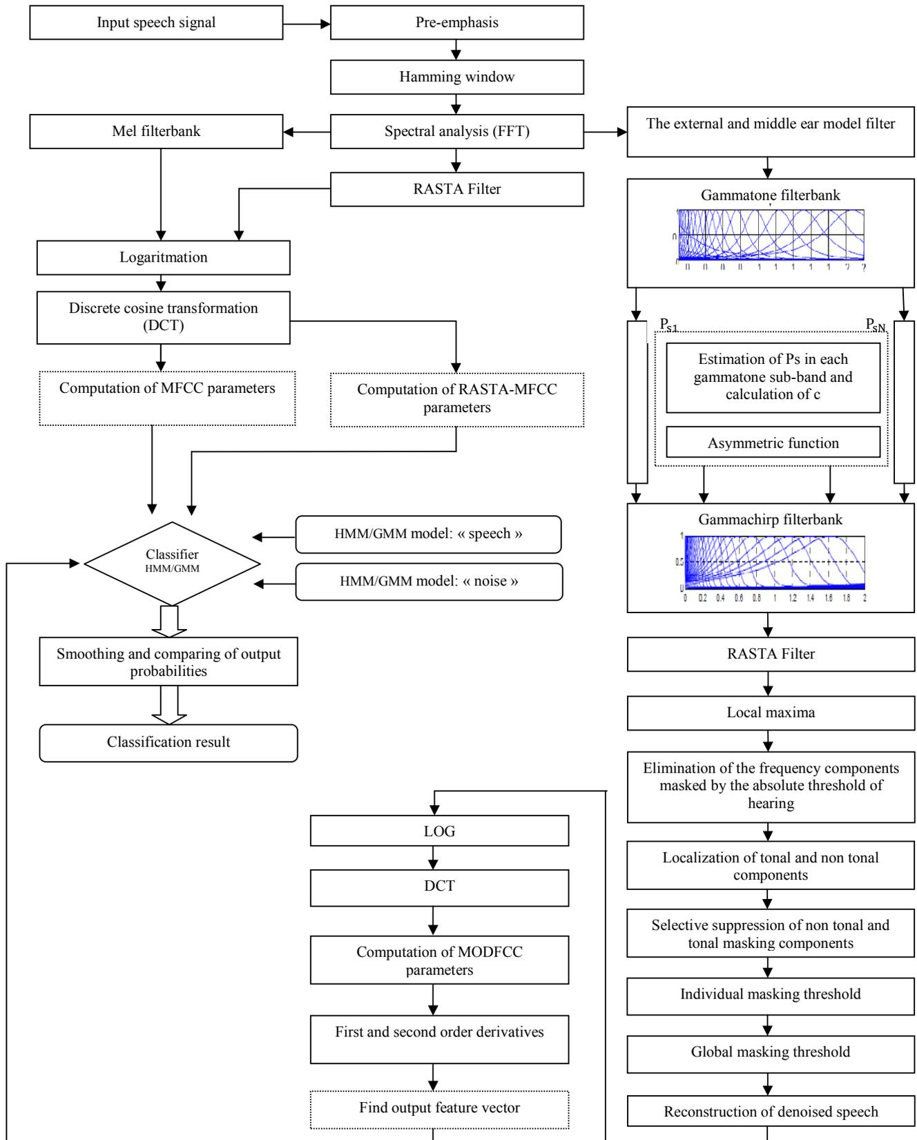
Fig. 2 The structure of MODFCC features extraction
