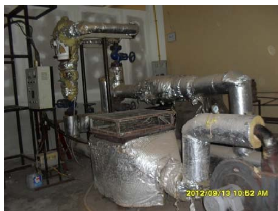
Fig. 2 The fluidized bed dryer used this study
