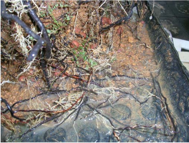
Fig. 5 Secondary roots spreading on membrane surface
