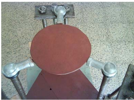
Fig. 2 A model of the 3 DOF Parallel Manipulator
