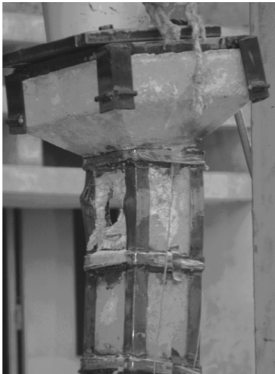
Fig. 20 Failure mode of eccentrically loaded strengthened column
