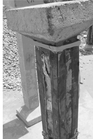
Fig. 21 Failure Mode of Eccentrically Loaded Column Strengthened using 40mm Angles
