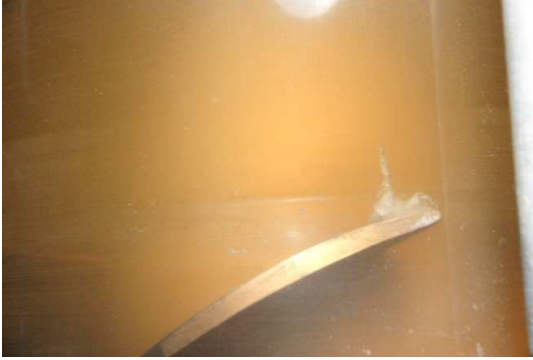
Fig. 13 Cavitation pattern under operating condition of No. 3-3
