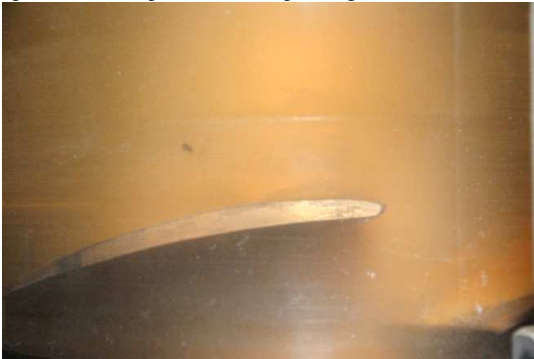
Fig. 2 Disappearance of cavitation under operating condition of No. 1-2
