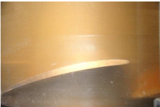
Fig. 3 Cavitation pattern under operating condition of No. 1-3
