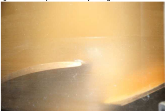
Fig. 4 Cavitation pattern under operating condition of No. 1-4
