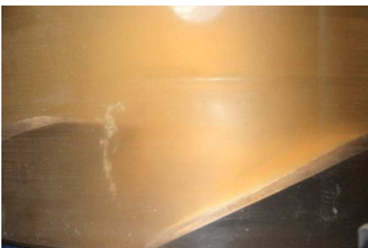
Fig. 10 Cavitation pattern under operating condition of No. 2-5
