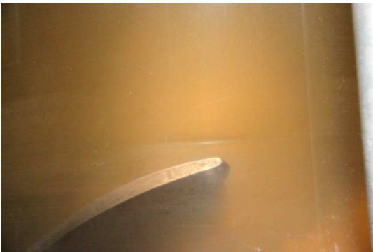
Fig. 14 Cavitation pattern under operating condition of No. 3-4
