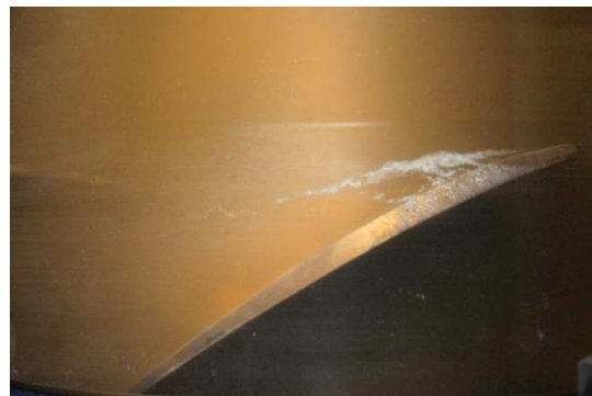
Fig. 12 Cavitation pattern under operating condition of No. 3-2
