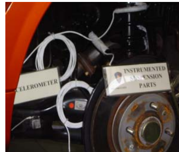
Fig. 2 Instrumented suspension system
