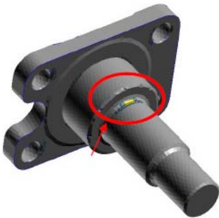
Fig. 1 Critical stress location
