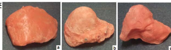
Fig. 2 Anthropomorphic phantoms representing the liver in (a) initial state cirrhotic, (b) intermediate and (c) advanced
