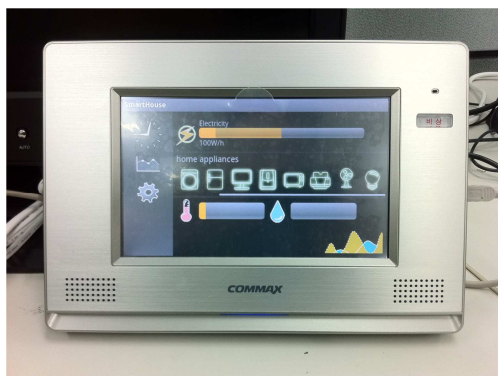
(a) Energy control wallpad
