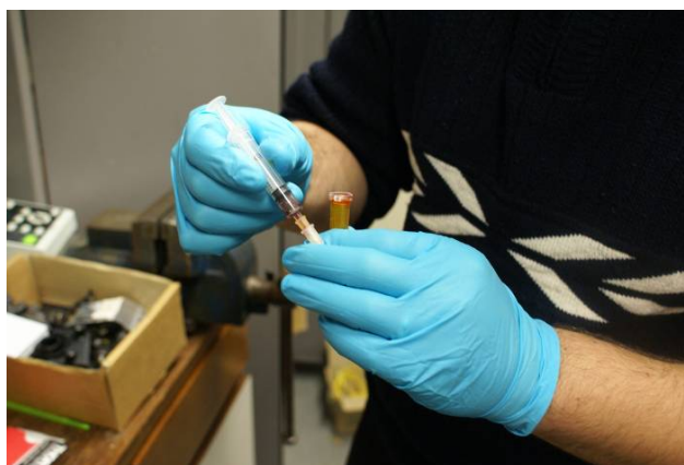
Fig. 11 Applying the fluorescent agent using a syringe
