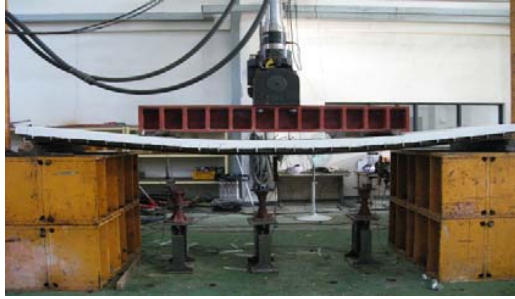
Fig. 3 Deflection under maximum loading condition
