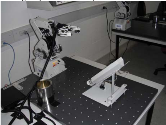
Fig. 7 Lab Volt 5150 robot with mounted gripper setup
