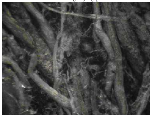
Fig. 5 Microstructure of fiberboard made of durian rind through latex with phenolic resin with the density of 800 Kg/m 3 at the ratio of 1:1 and 30x magnifying power
