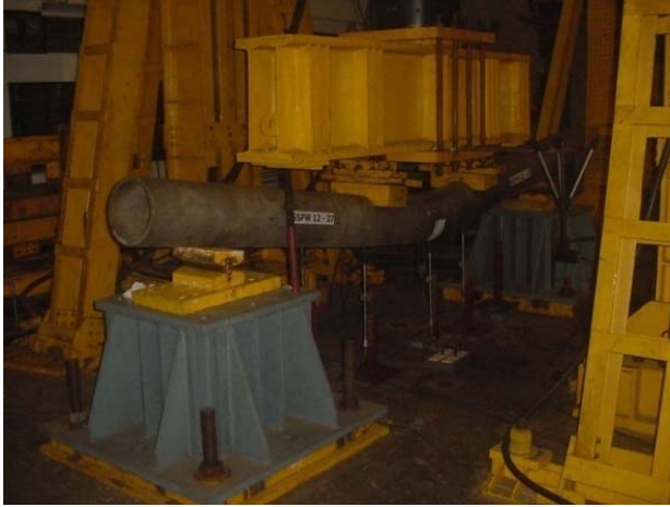
Fig. 2 Close-up view of monotonic fracture experiment
