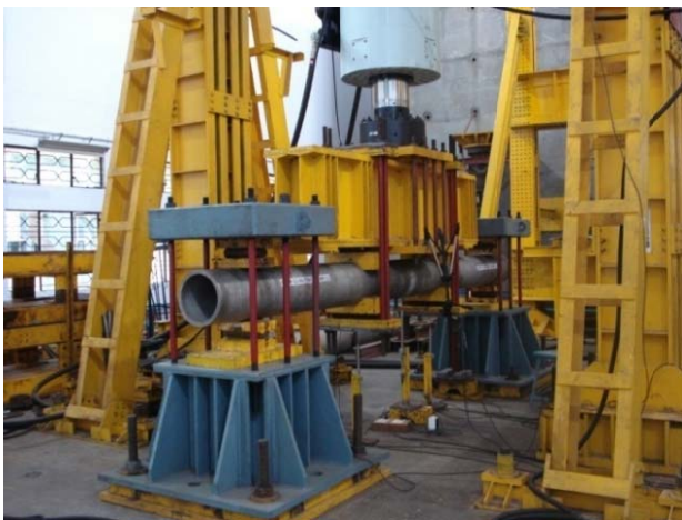
Fig. 3 Close-up view of cyclic fracture experiment
