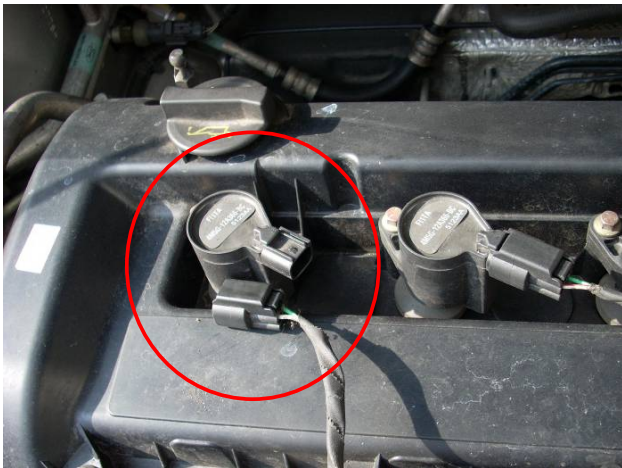
Fig. 10 Offline testing of ignition coil
