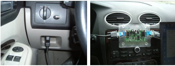
Fig. 9 OBD port (left part), OBD-II to RS232 adapter (right part)
