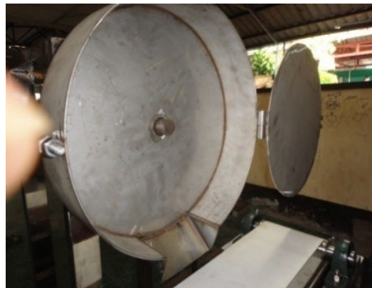
Fig. 4 The cover of sliced dish
