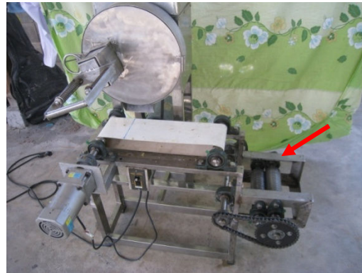
Fig. 3 The sliced cutting roller
