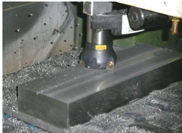
Fig. 2 Magnetic clamping of the workpieces
