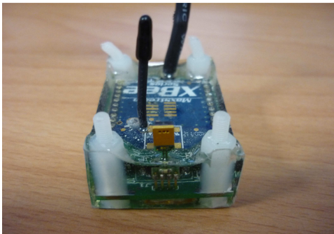
Fig. 1 A sealed but unpackaged STIM transmitter
