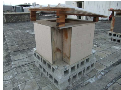
Fig. 5 Experimental group consisting of tiled exterior walls
