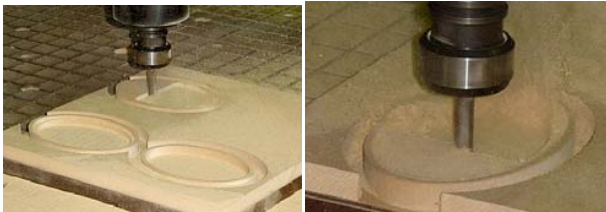
Fig. 9 MDF-board (Medium Density Fiberboard) machining of ellipses
