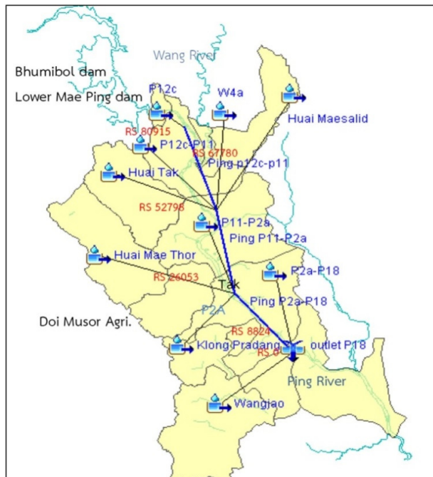
Fig. 3 Schematic map and location of lateral inflow from all catchments of the Ping River used in the HEC-HMS model
