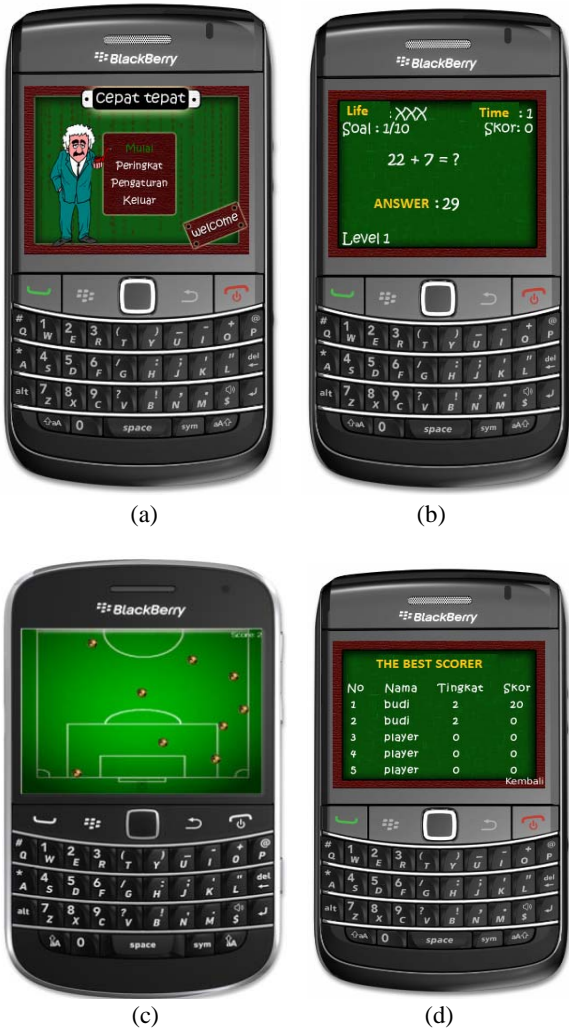
Fig. 5 Result of simulation using BlackBerry Simulator, Main form for starting and choosing games animation/mathematics(a), question in mathematics games (b) and example of ball games(c) and the best scorer stored in SQLite (d).
