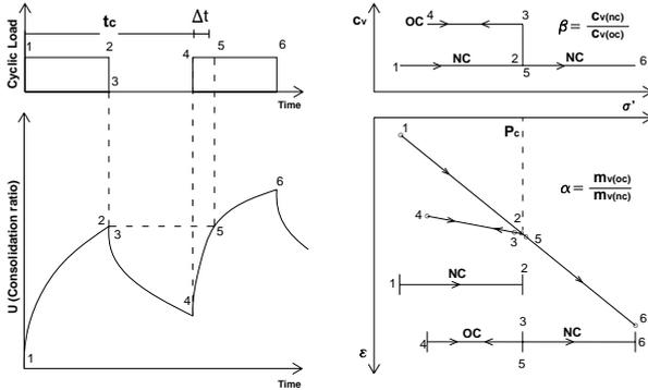
Fig. 1 Inelastic behavior of clay under cyclic load
