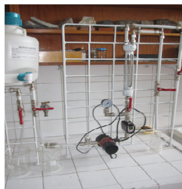
Fig. 5 Installation with vertical reactor to filter emulsions
