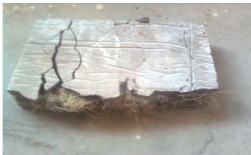
Fig. 5 Sisal fibre reinforced tested slab (3% fibre)
