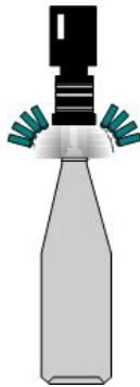
Fig. 4 The illumination of bottle finish
