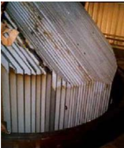
Fig. 4 Case of current circulation in the core
