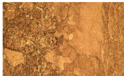
Fig. 7 TZ in the specimen welded at 2000 RPM (a second location)
