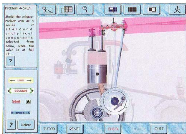
Fig. 5 Authoring a problem, showing the colored tolerance zones associated with machine element icons (beam and point forces in this case)
